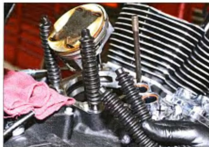
11 To protect the pistons and their rings, he fitted flexible plastic tubes over the cylinder studs.
