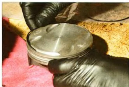
13 The piston rings were checked for correct end gap and then installed onto the pistons.
