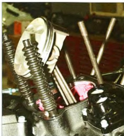
14 The new cylinder base gaskets were fitted over the cylinder studs. Then the pistons and their wrist pins were given a light coat of oil and were installed onto the connecting rods.
