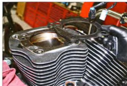
10 Mark pulled the head gaskets from the top of the cylinders.
