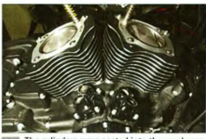
17 The cylinders were seated into the crankcase and the reassembly process started. To be continued...
