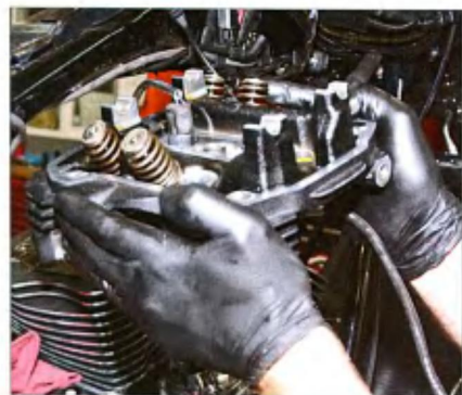
9 The cylinder head nuts were removed and the heads were lifted off of the cylinders.
