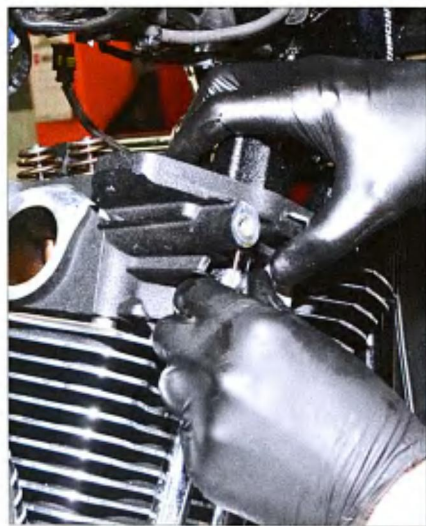
8 Mark then pulled the pushrod tubes.
