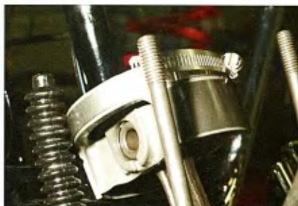
15 Large diameter hose clamps (Ideal No. 462) were used to compress the rings on the pistons. Next, the rags were removed from around the connecting rods.
