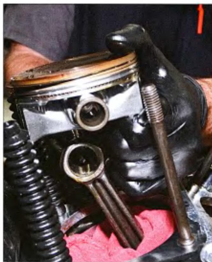
12 To prevent small parts from falling into the crankcase, rags were wrapped around the connecting rods and pushed down into the crankcase bores. The right-side wristpin keepers were removed, the pins pushed out, and the pistons were lifted off of the connecting rods.
