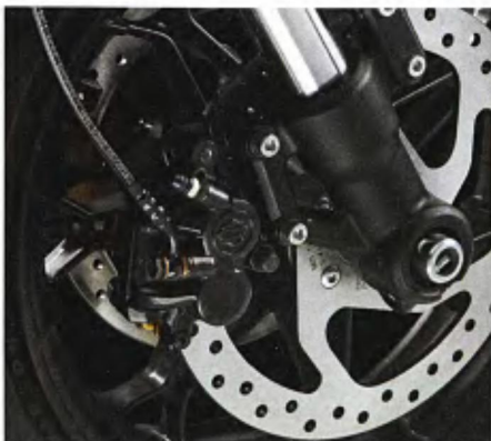
Dual disc brakes in the front and single disc in the rear, but all of them with 2-piston brake action. This ABS-equipped bike stops on a dime.
