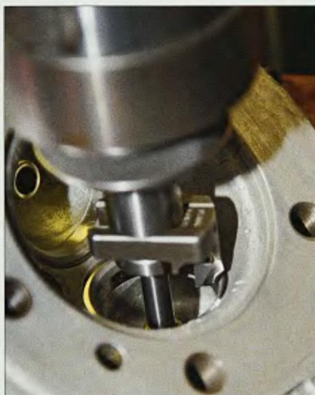
10 FSeats were first rough-cut then given a three-angle profile on the new seats.
