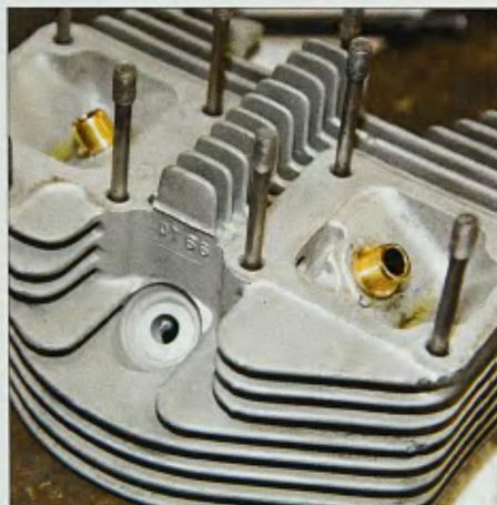
8 The shouldered bronze valve guides were pressed into the heads.
