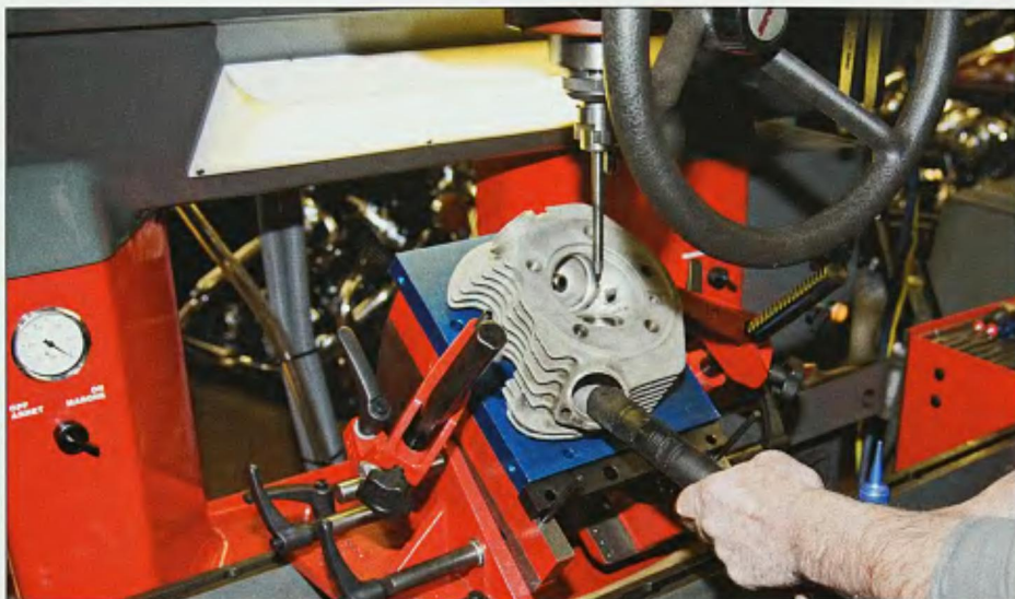
9 Andrew used a Serdi high-precision cylinder head machining center to finish the valve seats.
