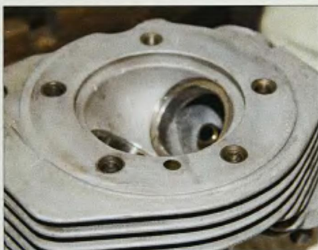
6 He then fitted the new valve seats into the heads.
