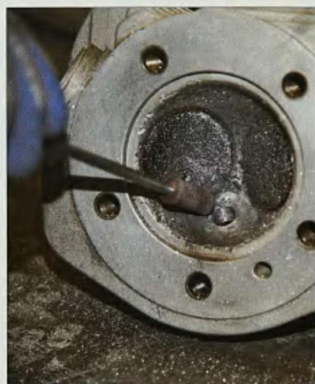
2 The rebuilding starts with cleaning the combustion chambers and inspecting all of the valves and their associated parts. To protect the valve seat areas and the cylinder head's ports, Andrew left the valves in the heads while he cleaned the carbon build-up in the combustion chambers.
