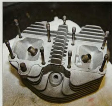
3 He finished cleaning the heads in two steps. He first washed them in a chemical parts washer then bead blasted them with non-abrasive ceramic media.
