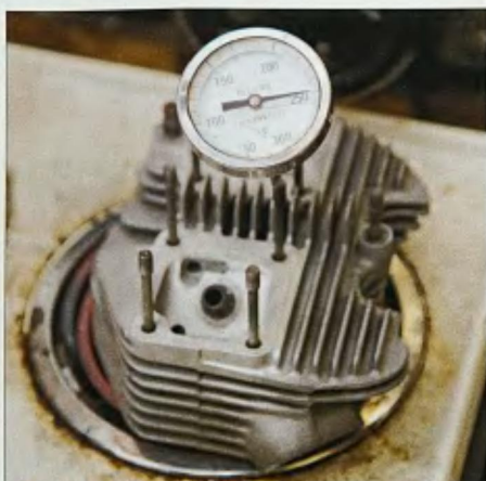
5 After he removed the old valve seats, Andrew heated the aluminum head casting on an electric range.
