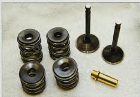
7 He used shouldered bronze valve guides, nitride valves, and spring kits.
