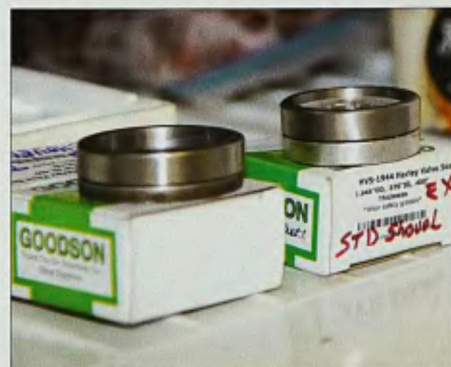
4 The new valve seats are made from cast iron, which works well with the aluminum heads and steel valves.
