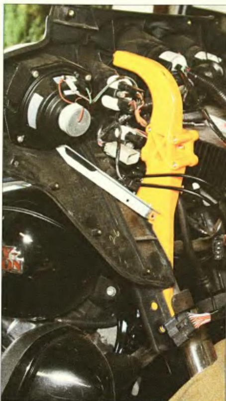
9 Even though it has a larger cross section, the Strong Arms fit right where the factory bracket came out of.
