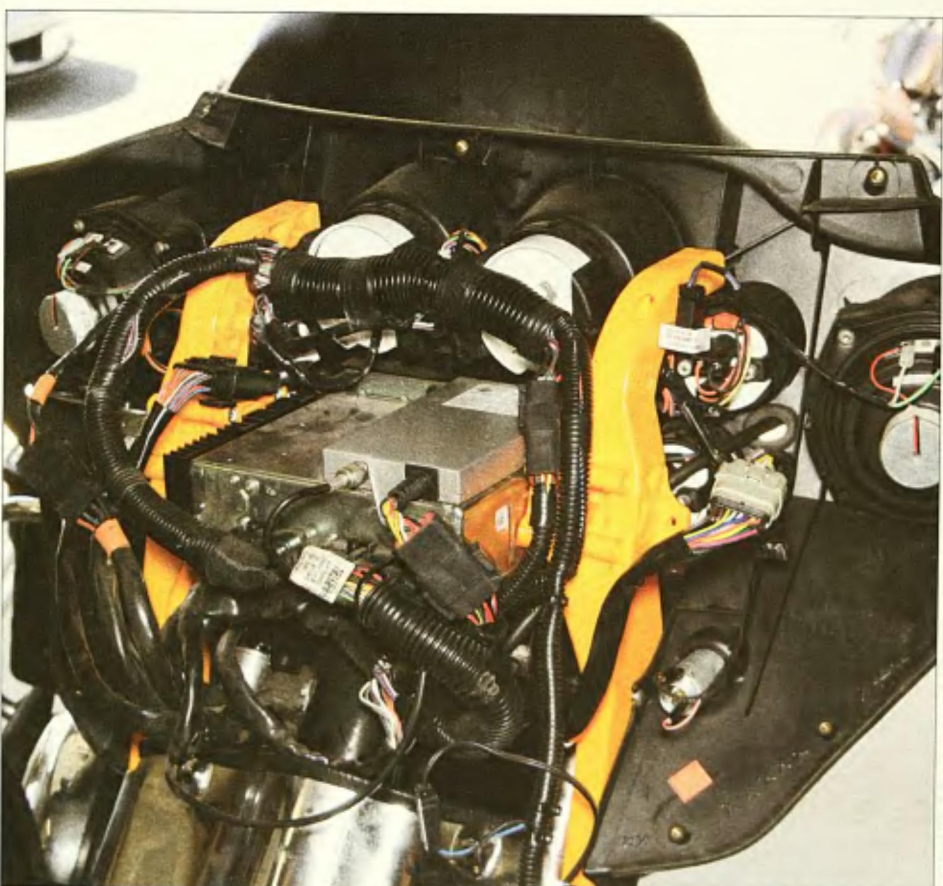
11 Once both of the new brackets were in place, we tightened all of their mounting bolts. There are six on each side: two at the inner fairing, two at the radio and two at the triple trees on the fork. Installing the fairing, completed the job. The finished installation was very tight when compared to what we started with.
