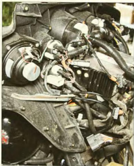
7 We had to unplug a couple of wire harnesses to get the factory bracket out.
