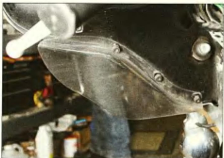
3 On the backside of the fairing, there are five Torx and Allen bolts that run down each edge of the fairing to remove.
