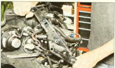
8 We removed and replaced the brackets one side at a time. The factory brackets are very stout except at their upper end.
