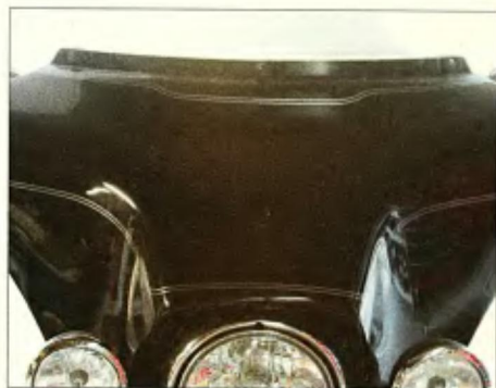
2 Removing the outer fairing starts at the windshield, there are three Torx screws to remove.
