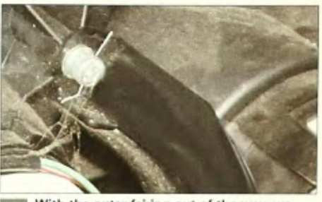
4 With the outer fairing out of the way, we saw that the upper ends of both of the fairing mounting brackets were broken off.
