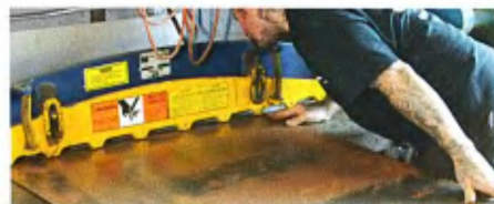
Tony runs a large piece of sheet metal through his stomp shear to cut the strip that will give the tank its three-dimensional look.
