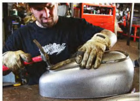
The piece is then hammered gently into the tank's opening to see how it fits.
