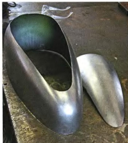
One half of the gas tank with its top cut out sits on the work bench awaiting Tony's special treatment.
