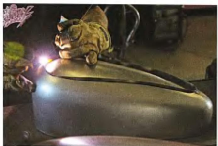
Once everything fits, the parts are welded together.
