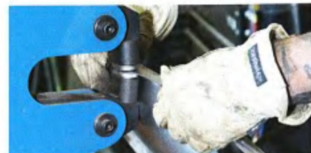
A shrinker-stretcher makes sure the part gets its proper radius.
