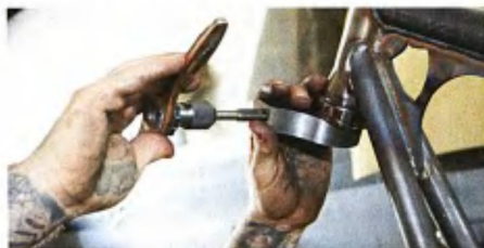
The triple trees have been machined and are getting their proper threading for the bolts that will hold the Harman front end.
