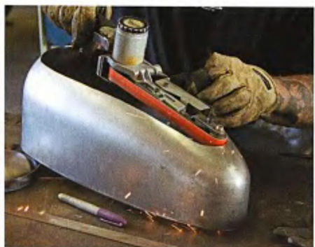
Additional adjustments are made with a special grinder.
