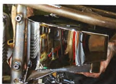
This oil tank is yet to undergo some modifications, but the battery is probably going to stay in it.
