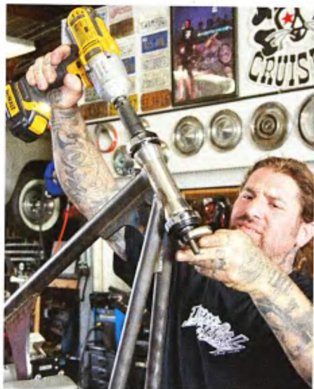
Tony assembles the neck for an initial bearing and fork stop check.
