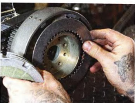
Clutch plates are installed so Tony can check their play.
