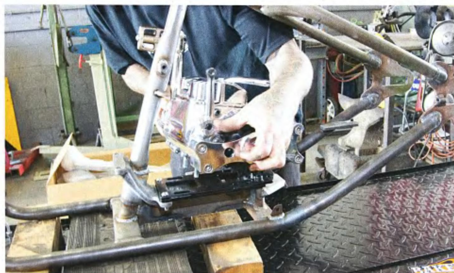
The mock-up of this chopper begins with Tony placing the Baker 4-in-a-6 transmission into the stretched Paughco frame.
