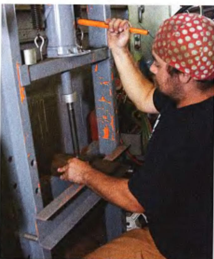
Gnomie presses the neck stem into the lower triple tree.
