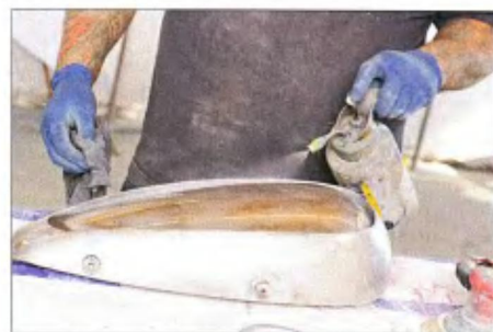
Spraying and wiping down the tanks with lacquer thinner ensures that there's absolutely no oil, slag, or any other contaminant left.
