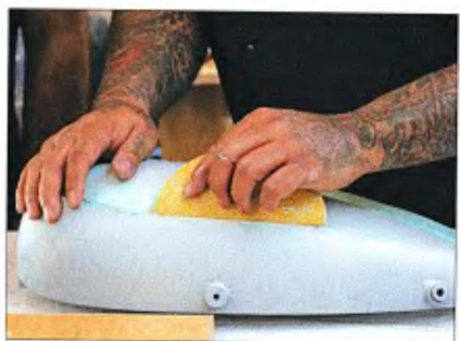
Once the bondo is spread evenly over the tanks seams, Manny sands it all down at least twice, using finer and finer grits of sandpaper.
