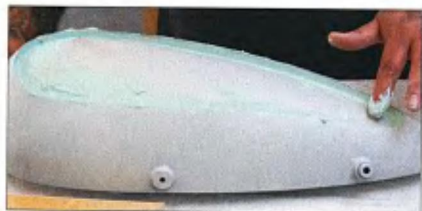
Manny spreads the lightweight filler onto the tank's groove to keep the area from rusting or otherwise deteriorating.
