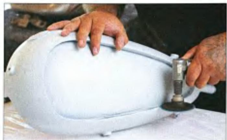
After the primer has dried, Manny uses the grinder to smooth out the edges.
