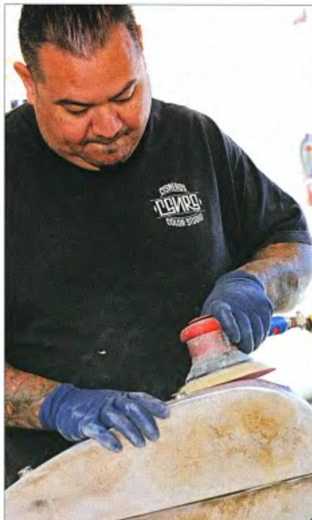
He then sands the tanks down with 80-grit paper to remove more leftover dirt or rust.
