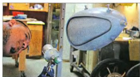
Then the sealant is sprayed on. Manny covers the tanks with two layers, just to play it safe.
