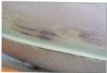
Though smooth as a baby's bottom now, the tank will get sanded a few more times and receive two more layers of primer before Manny is ready to paint everything.
