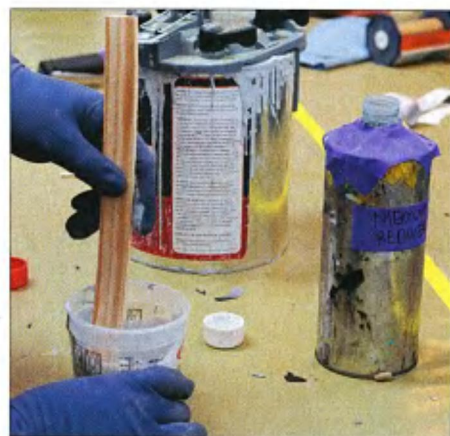
The next step is spraying the primer-sealer. Here Manny prepares enough to cover both tanks, mixing the primer with epoxy hardener.
