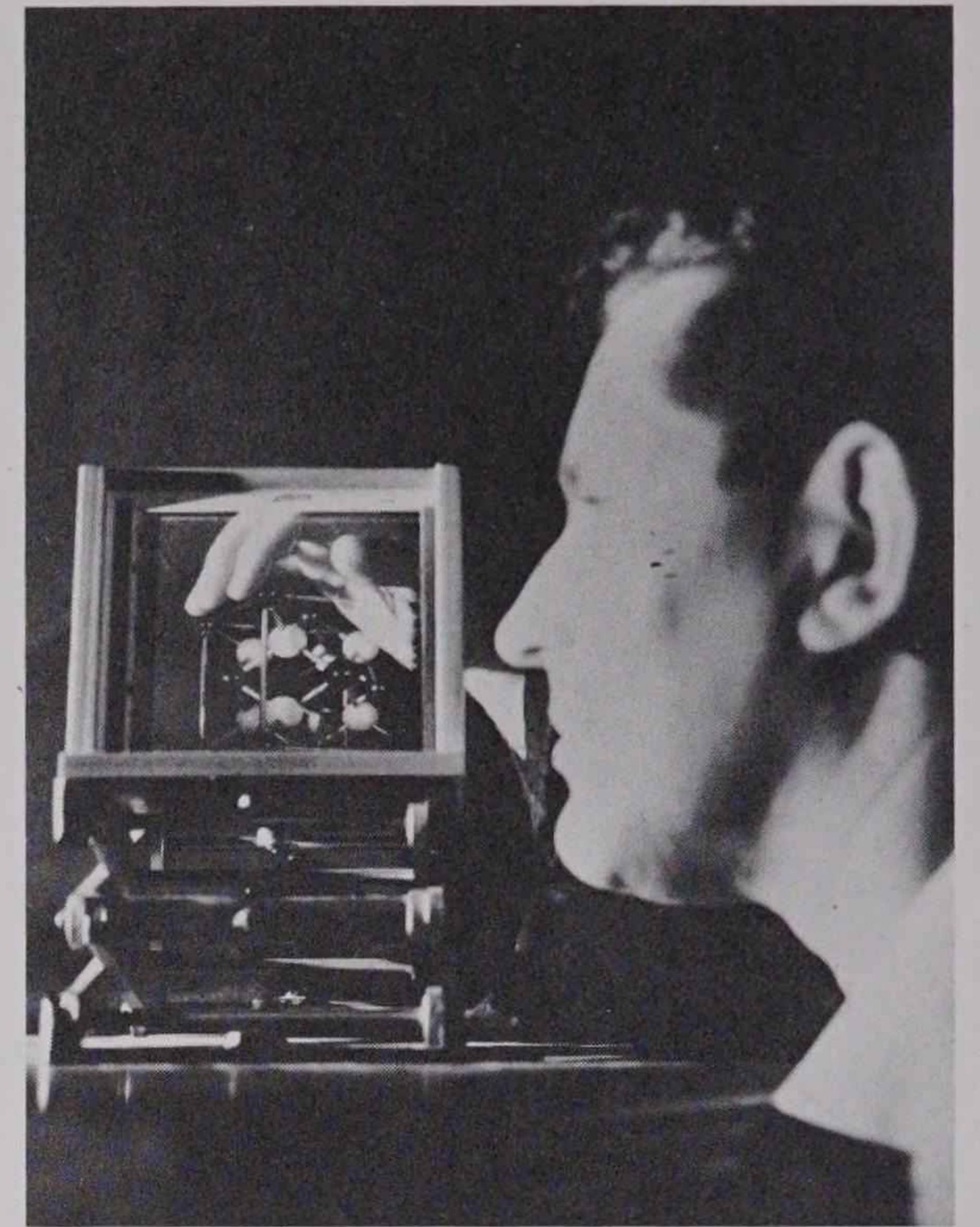
RCA Laboratories personnel engage in various types of holographic research. Left: A red laser beam is used to project real images of a Schubert figurine and music sheet. Center: A researcher adjusts a lens to produce a hologram at its focus. Right: A technician appears to hold a model of a crystal behind a window. The window, however, is a transmission hologram, and the model is only a three-dimensional image.
