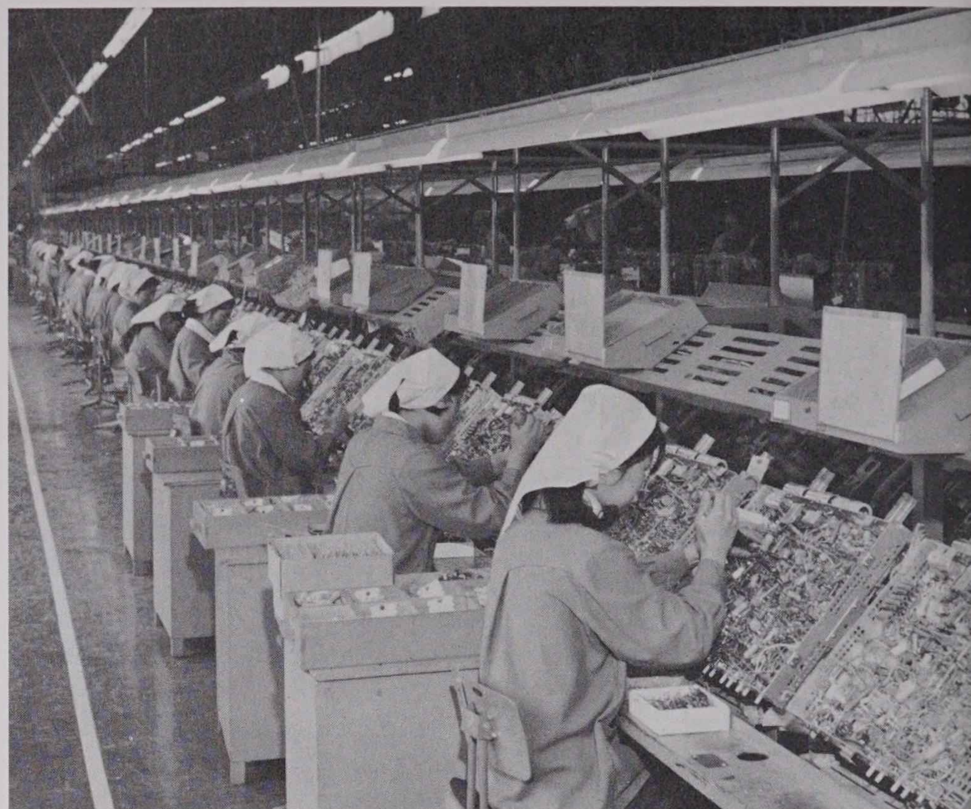
Workers assemble color television chassis at the Tokyo Shibaura Electric Company, the largest manufacturer of color sets in Japan.
