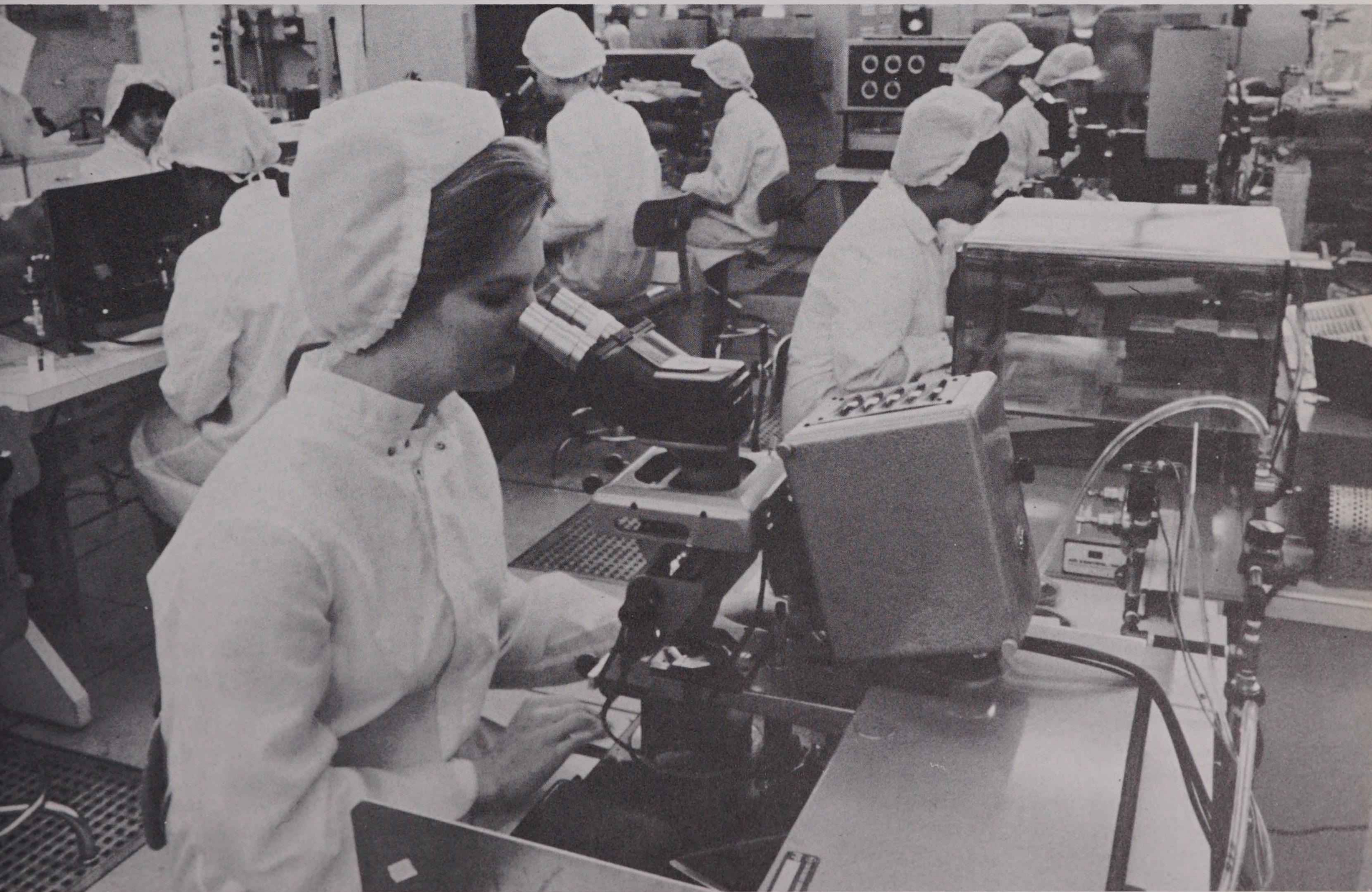
Microscopes are used to inspect a wafer of silicon on which have been etched a number of tiny integrated circuits.
