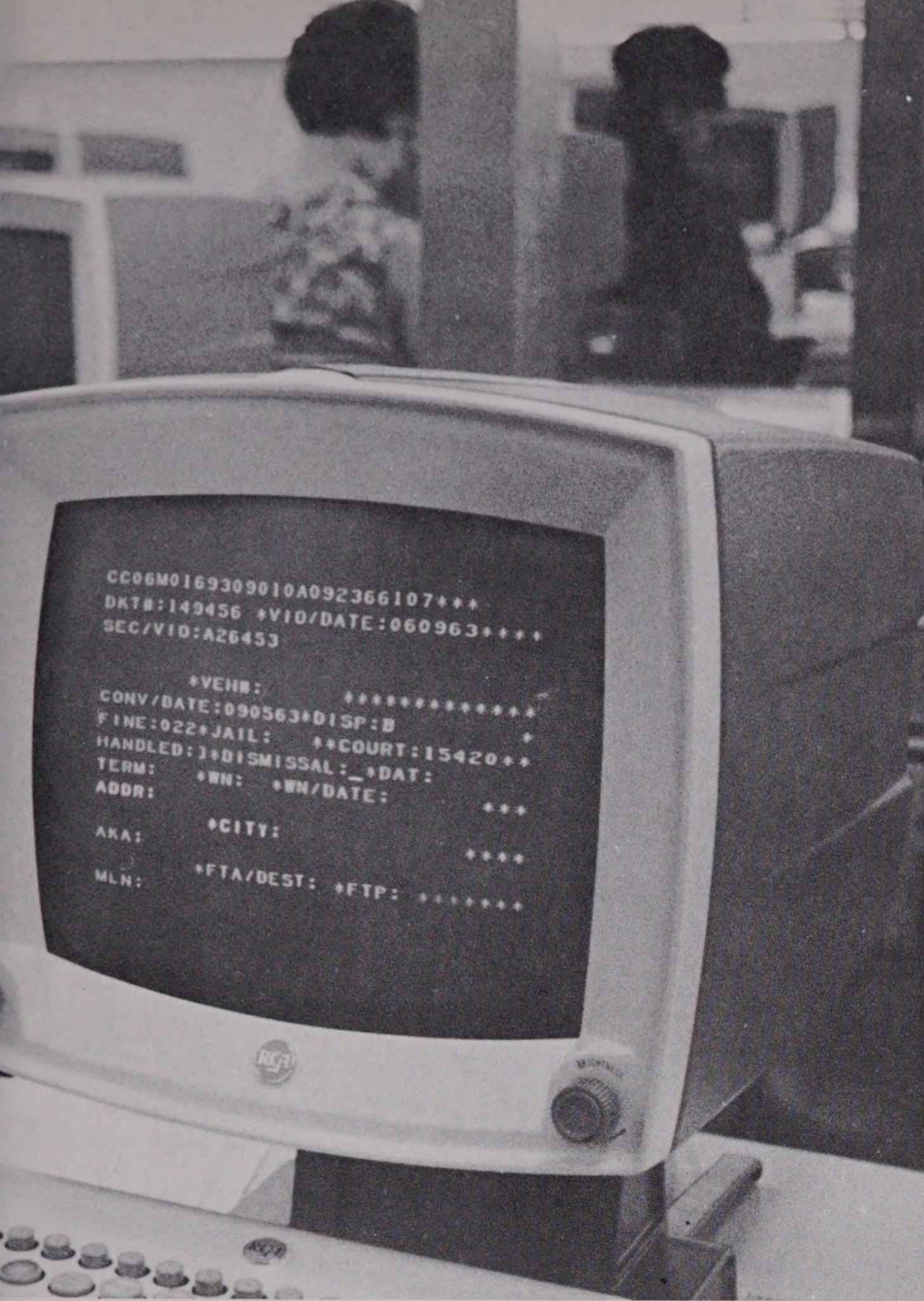
Motor vehicle records are displayed directly from a data bank onto the screen of a video display device. The system is part of the California Department of Motor Vehicles huge computer-communications network.
