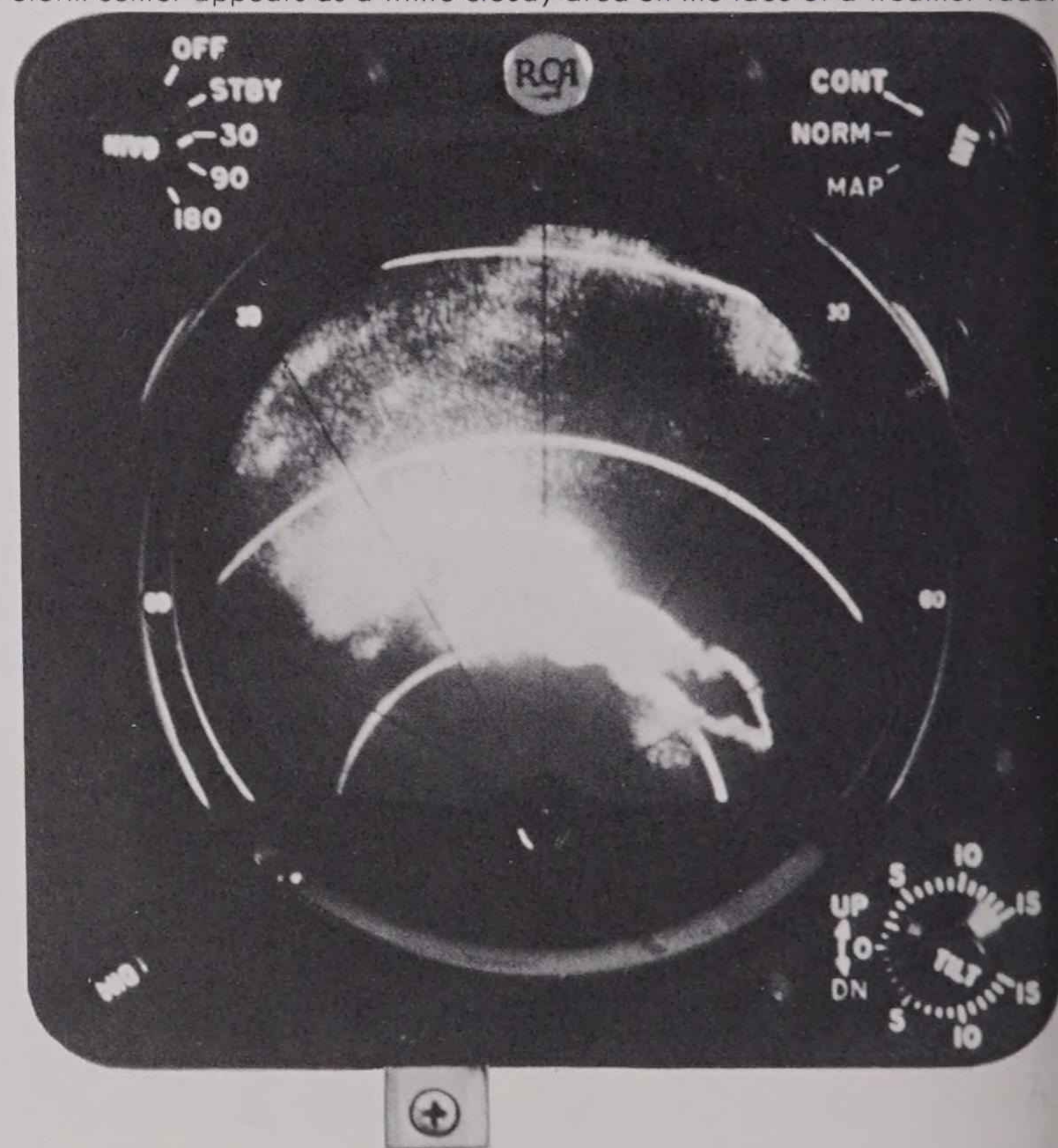
Storm center appears as a white cloudy area on the face of a weather radar.
