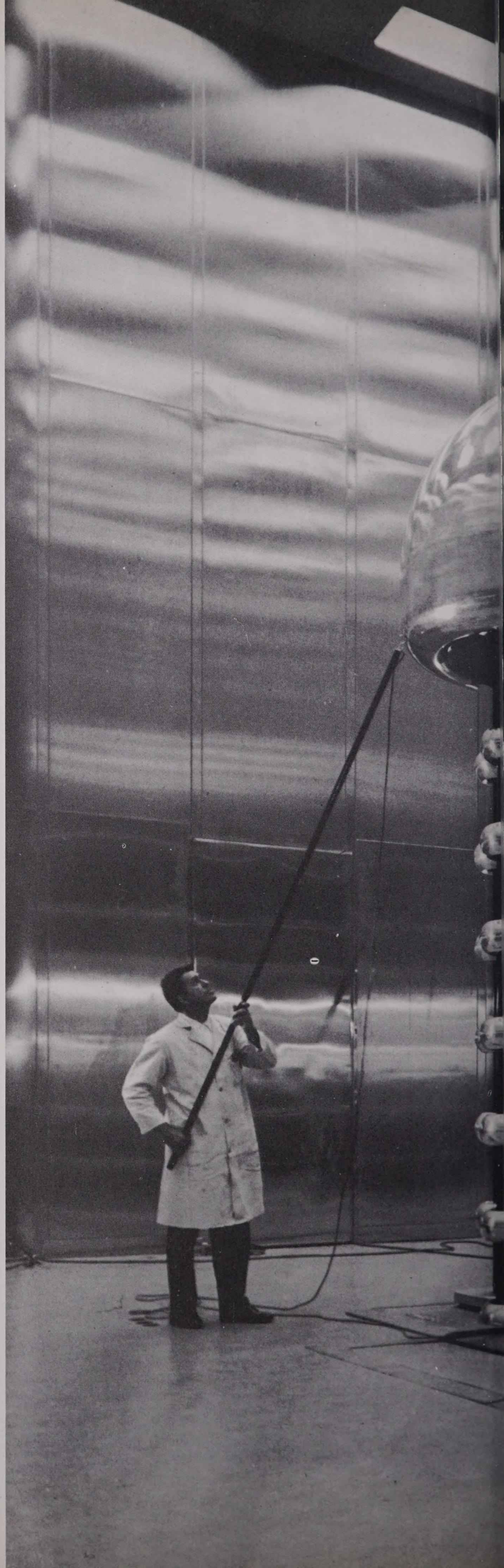
Accelerators for U. S. Steel's electron microscope drive its electron beam at nearly the speed of light.
