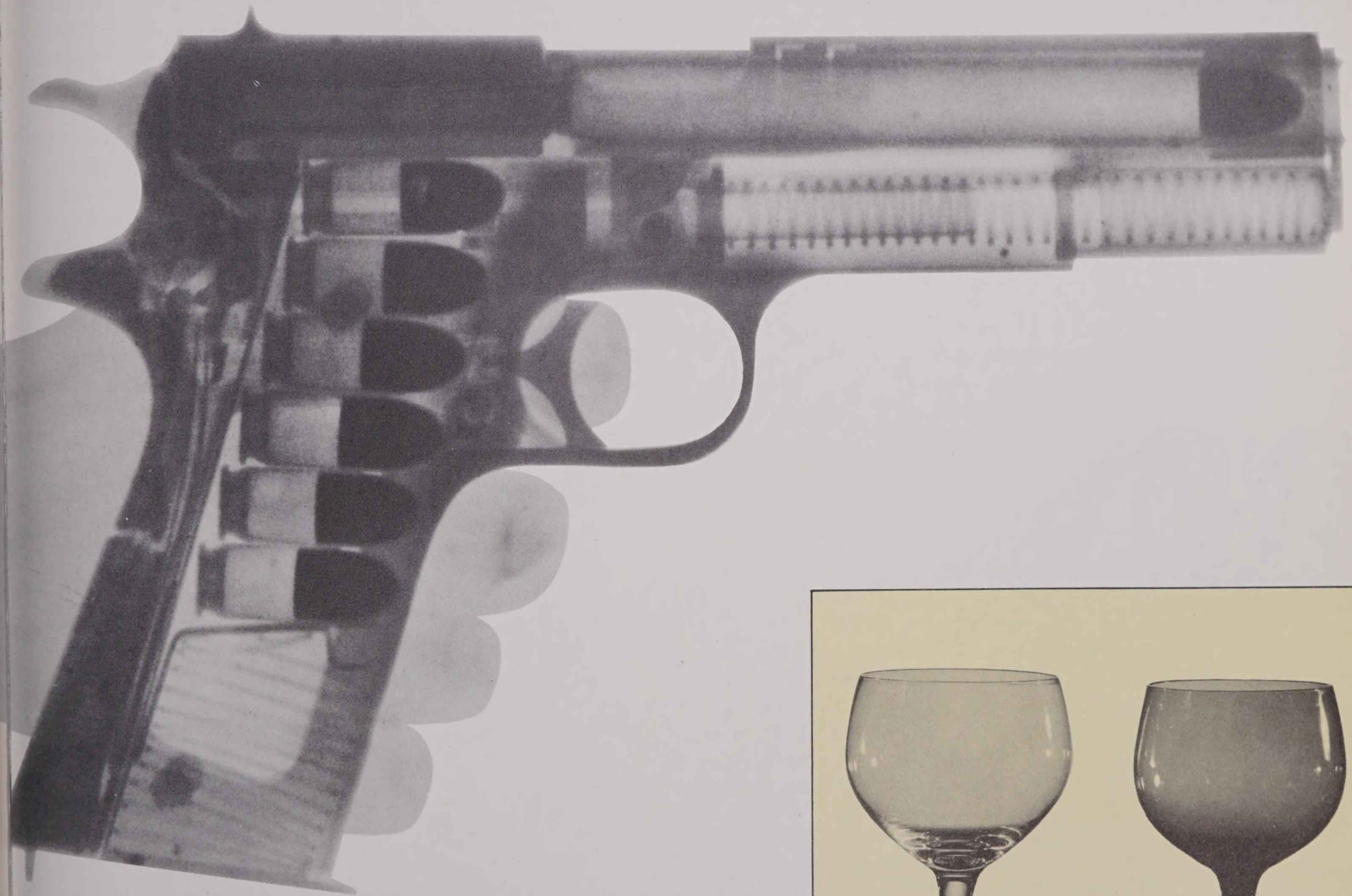
'flash X-ray' photograph of a pistol at the moment of firing.
