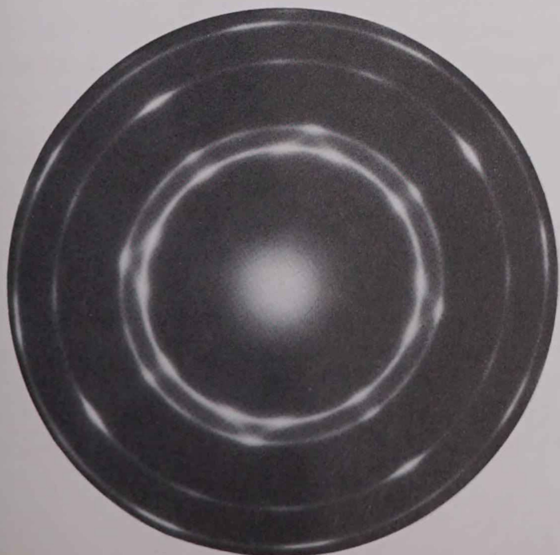
Atomic structure of titanium (top) and nickel chromium crystals are revealed in these X-ray photographs.
