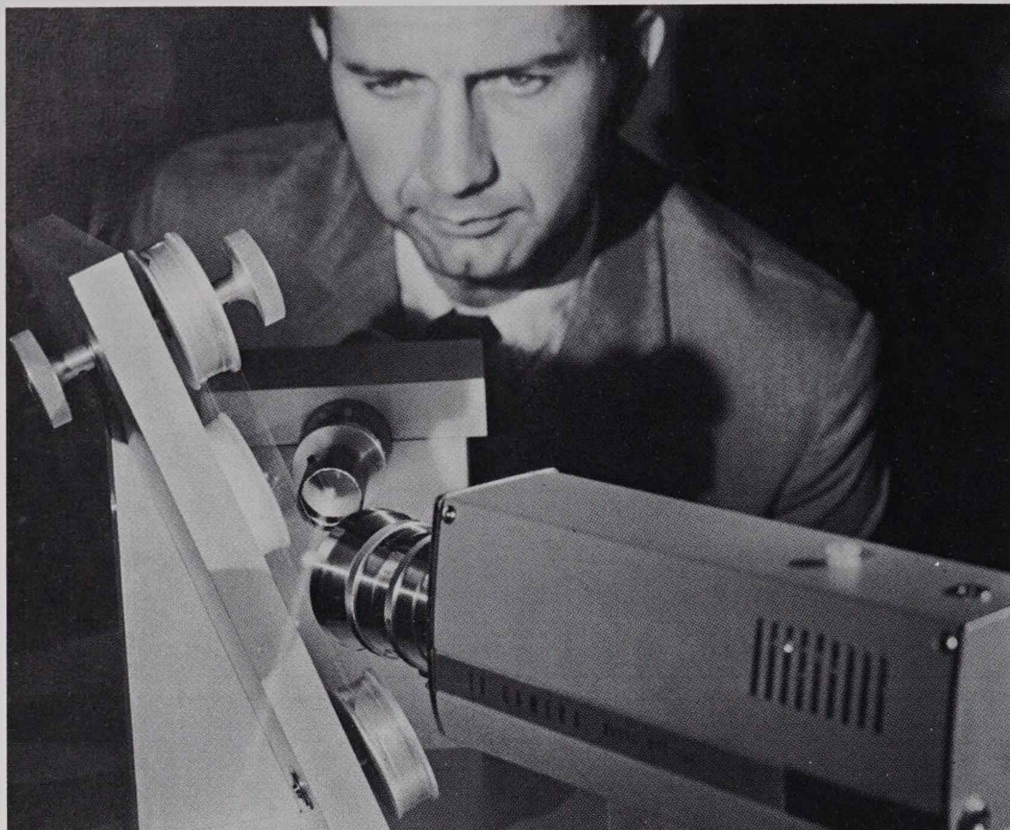
RCA's color TV tape player system is based on laser technology. Here a low-power gas laser (center) sends a beam through the holograms on a vinyl tape. The result is picked up by the TV camera and deciphered to produce color pictures on a standard television receiver.
