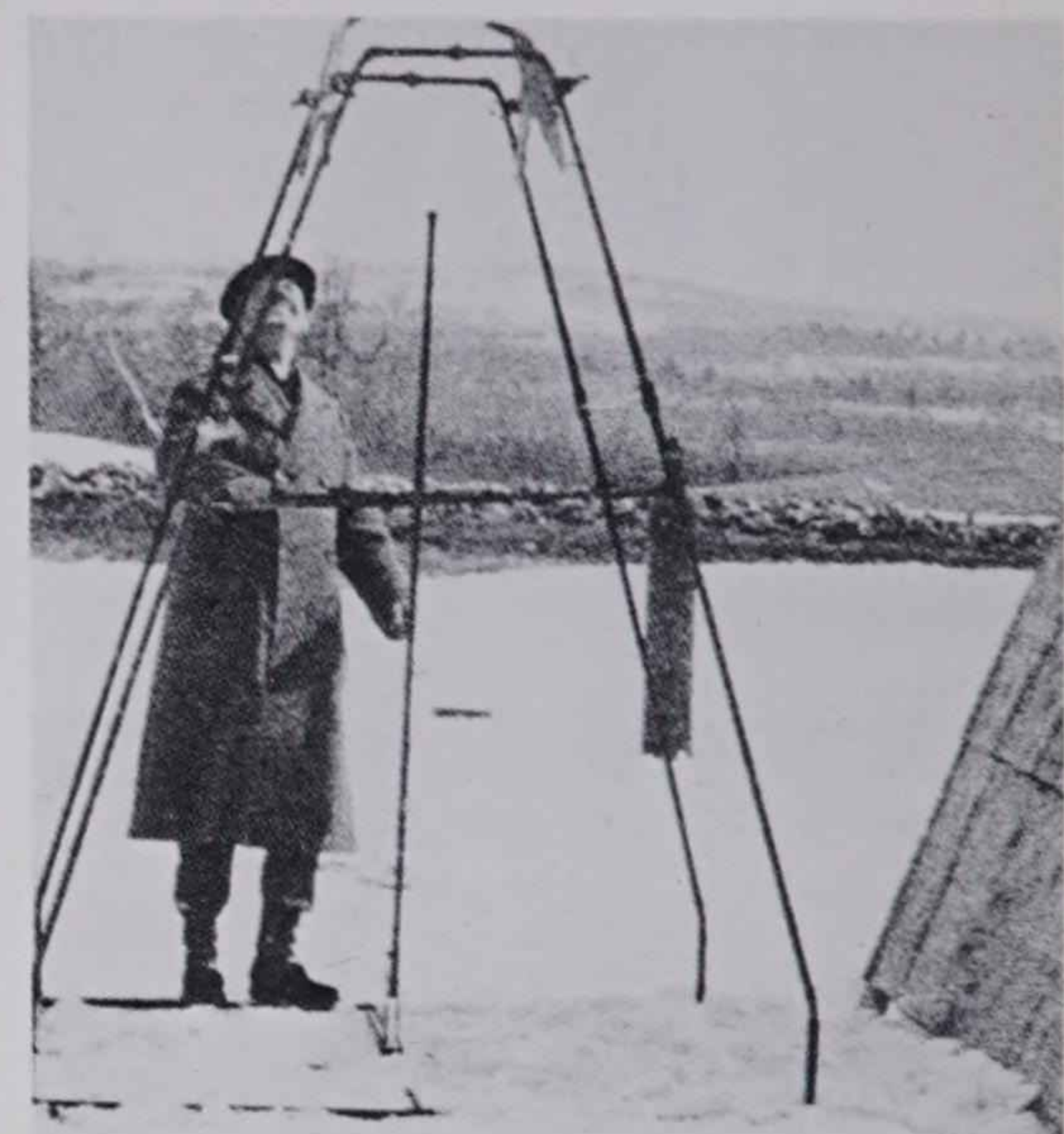
This frame supported the rocket during its first launch at Auburn, Mass.
