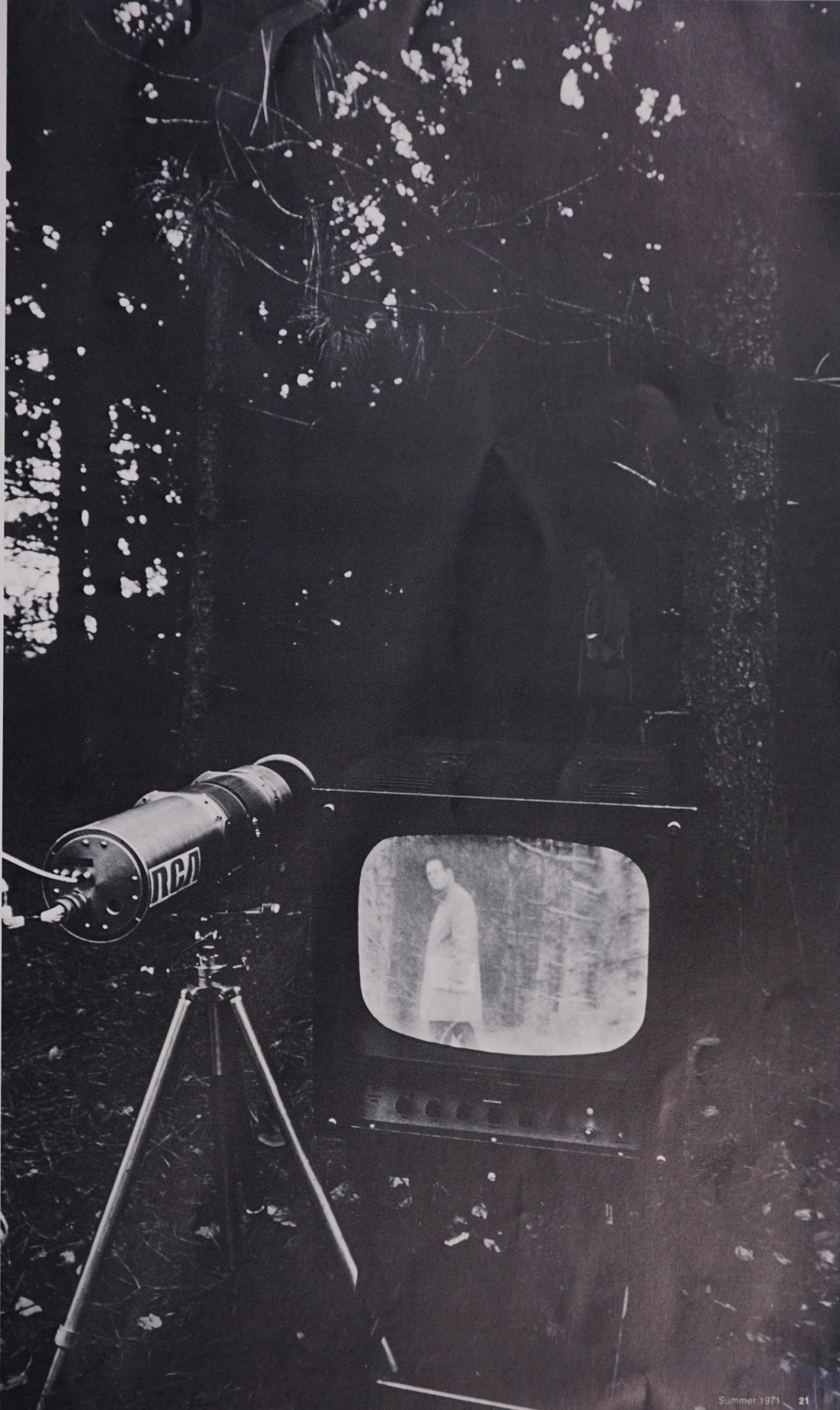
(Right) The unaided eye can barely discern the man in the background; however, the low-light-level TV camera intensifies the image, which can be seen on the screen in the foreground.
