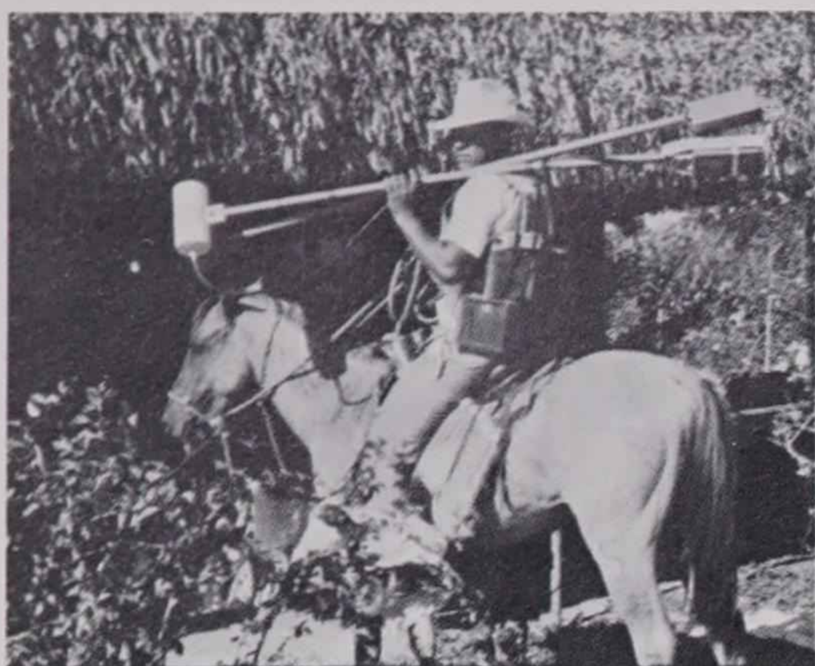
Portable cesium magnetometer is moved to a site near San Lorenzo, Veracruz, Mexico.
