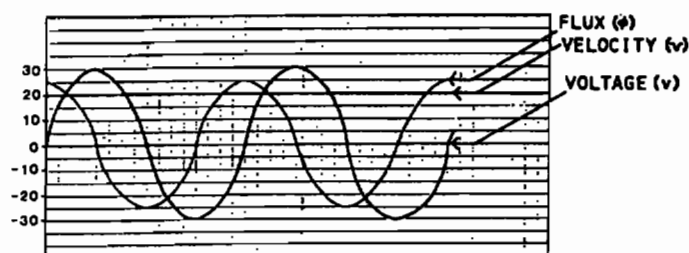
TWO CYCLES OF FLUX AND VOLTAGE COMPARED WITH TANGENTIAL VELOCITY IN STANDARD GENERATOR
