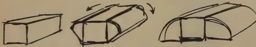
Portable home to be built to SeaLand trailer specifications, fastenable to bolts in twelve concrete pylons. These would be transportable by sea, rail or truck. The pylons could be constructed at any number of sites, the house being transported from one to the other.
