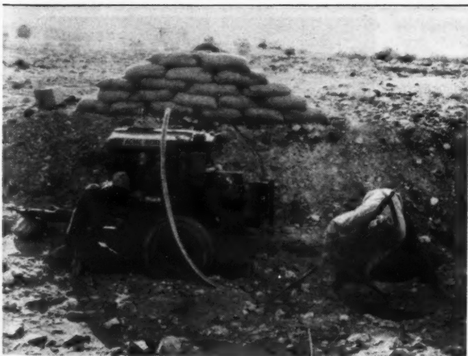
The big generator cost $315 for three weeks. To cut the noise we stuck it in an arroyo 250 ft. from the camp (required 3/8" wire), built a barrier of
