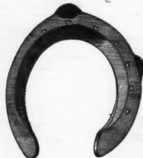
A right front shoe with nailless and narrow inner branch for a base-wide hoof. Suitable for horses that strike anywhere from inner toe back to the quarter.
