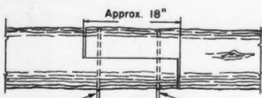
Drift pins to extend into second log below SPLICING LOGS
