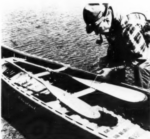
Because the flat surface of the paddle blades rest on the shoulders, this type of yoke is one of the most comfortable. Photo by Eleanor Riviere.
