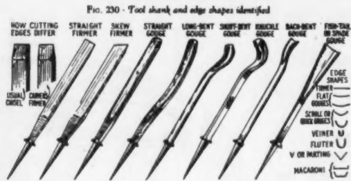
FIG. 230 - Tool shank and edge shapes identified
