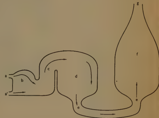
Figure 10.8 Two-chamber draught kiln (section)
