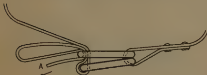
FIGURE D-12.—Quick-release loop.
