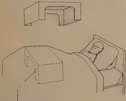
FIG. 15-1. A cradle to keep bedclothes off legs and feet, made from a cardboard carton.
