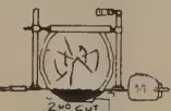
Second Cut—Use sawn surface as roller guide. Raise roller assembly and remove BOTTOM SLAB.
