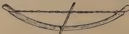
Fig. 54.—Spanish Windlass (for bending wood)
