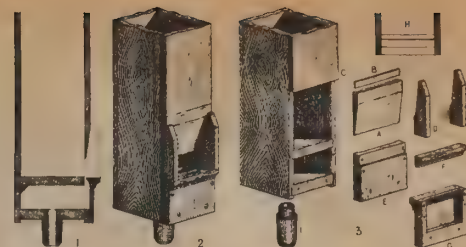
Wooden pipe of a Principal or Open Diapason , 16 ft.
