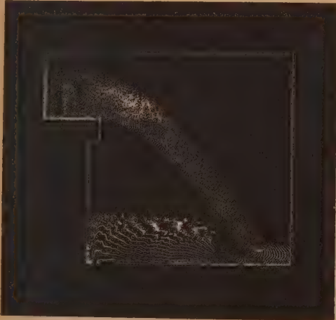
10. Simulated waterfall spills over the edge of a cliff and splashes into a pool in this computer experiment performed by John P. Shannon at the Los Alamos Scientific Laboratory as part of a study of dynamic behavior of fluids with the aid of numerical models.
