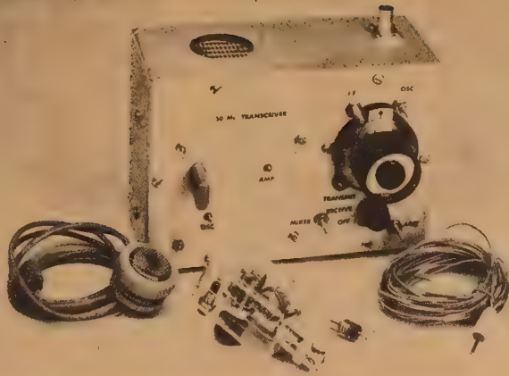
Fig. 19-6—The 50-Mc. transistor station, complete with microphone, battery and antenna system, weighs in at under 3 pounds. The antenna coupler built in a small plastic parts box is used with random "long wires." Coax-fed antennas connect directly to the BNC fitting on the top of the case.
