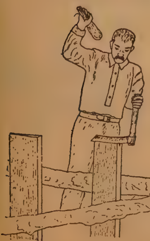
Fig. 49.—Splitting with a Froe
