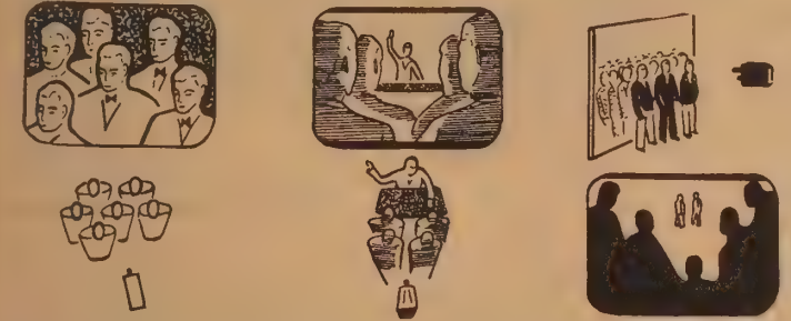
CROWDS can be simulated by using selective viewpoints (left) and carefully positioned subjects crowded together along the lens axis (centre). Also by augmenting subjects with a background of a crowd scene (moving back-projection, photo-mural, painted cloth) or using dummy or cut-out foreground figures (right).
