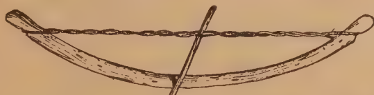
Fig. 54.—Spanish Windlass (for bending wood)
