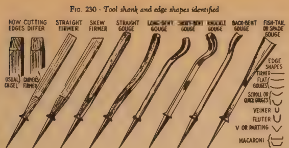
FIG. 230 - Tool shank and edge shapes identified
