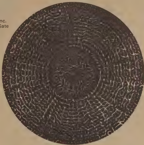
A sonorous figure produced by piezoelectric excitation. The triangle measures 24 cm along each edge. Steel plate. Frequency 875 cps.
