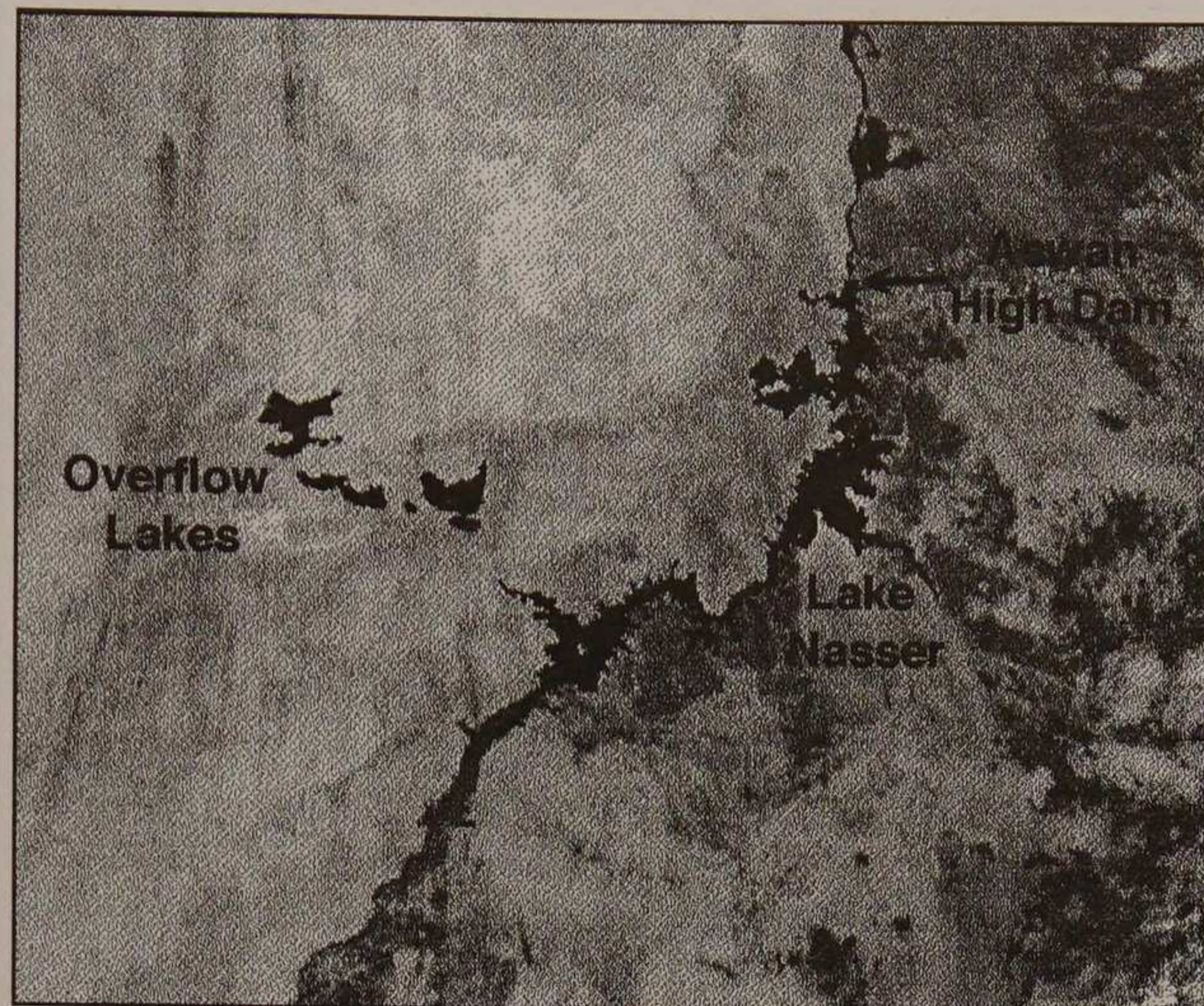
Figure 10. Satellite image of the Nile River around Lake Nasser and Aswan High Dam. The exceptional rainfalls in the Nile River Basin after c.1994 slowly filled Lake Nasser to capacity, for the first time in its 35-year history. The excess waters were diverted into the Toshka Depression, out in the open Sahara Desert, where four giant overflow lakes were created for the first time since the Sahara Wet Phase of c.5000 BCE. (From the MODIS imaging spectroradiometer, NASA, 10 October 2000.) http://visibleearth.nasa.gov/cgi-bin/viewrecord?6506
