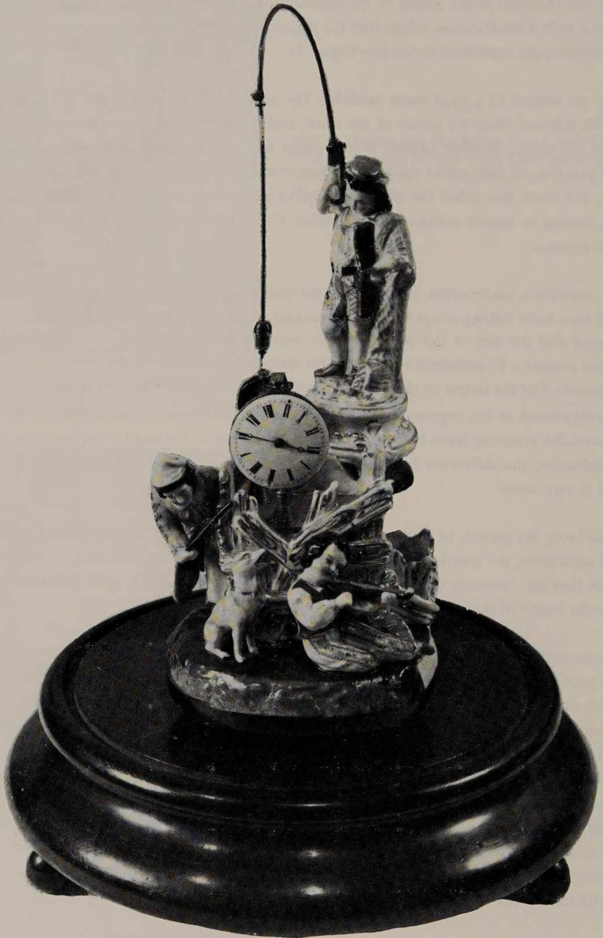
Fig. 3. Porcelain Conical Pendulum Clock, circa 1880. The fisherman's line is rotated by a \frac{3}{16} in. diameter wheel of a special watch movement.
