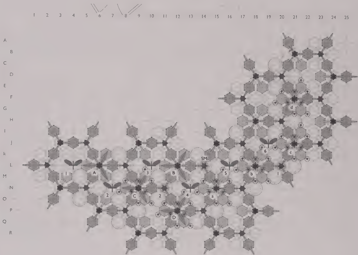
Figure 3. Plan of Sentient Chamber showing modular combinations of structural scaffold components integrated with mechanisms and sensor clusters. The structural design follows diffusive crystalline forms.
