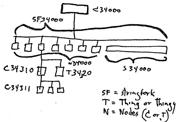
**NODE LOADER AND BOOTSTRAP.** The Node Loader calls in specified program nodes, as listed in the current stuff. The Bootstrap brings in the Node Loader, at startup or when core really has to be purged. Node loader also sorts its needs for single tape pass (if tape system). NODE LOADER INCLUDES NODE SEARCH TECHNIQUES.
