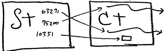
SWAP ROUTINE. Clobber the crums not needed, searching node numbers to determine; push what must be saved, or leave it in core.
