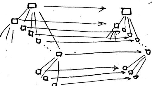
The Dual Tree Structure permits complete relocatability, context and program switching in an open-ended manner. The Spec. Tree tells what is where in the Lookup Tree, and where the LU tree elements are in core, if they are in core.
