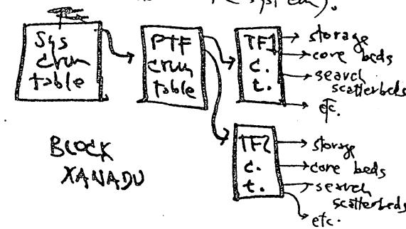
The same Rule of Order, however — of each functional block minding its own housekeeping pointers — seems a good system to build from.
