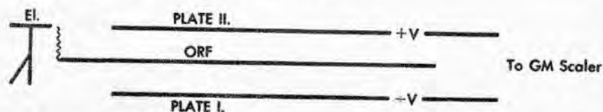
Fig. 8. Arrangement for the measurement of the excited OR energy field (ORF) in high vacuum. The deflection of the leaf of the electroscope indicates the strength of the OR energy field
