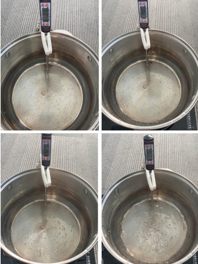
Water at different temperatures. Top left: 50.1°C; top right: 79.0°C; bottom left: 92.7°C; bottom right: 97.5°C. All following images were made by Lau Kai-yiu and the author's team.
