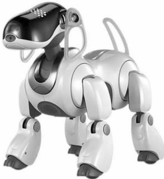
Figure 4. The Sony AIBO Robot: Main externally-oriented sensors are camera; infrared distance sensor; microphone; tactile sensors on head, paws, back and chin. Actuators include speaker, joint motors, and LED's on its face and back
