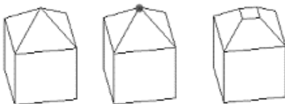
Figure 8. A capped cube (at left) is redisplayed with a highlighted “top” point (at center). After the solid is truncated at the suggested vertex we obtain the shape at right.
