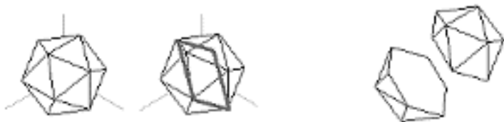
Figure 5. An icosahedron, redisplayed with a “slicing rectangle” at center. Note that the upper right vertex of the highlighted rectangle is one of the hidden vertices in the view at left. At the right, the two resulting halves of the sliced icosahedron.
