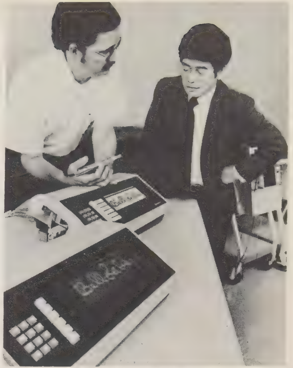
Visual communications over ordinary telephone lines is in the works. At Bell Labs a Flat-Screen video device can be used to transmit handwriting instantaneously.
