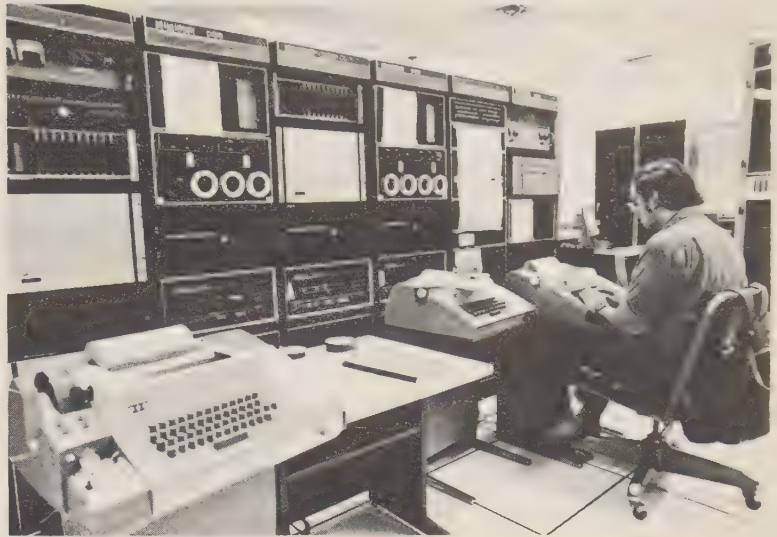
Shown here are four of the 16 PDP-11s tied together by CMU's multi-mini-processor system C.mmp.
