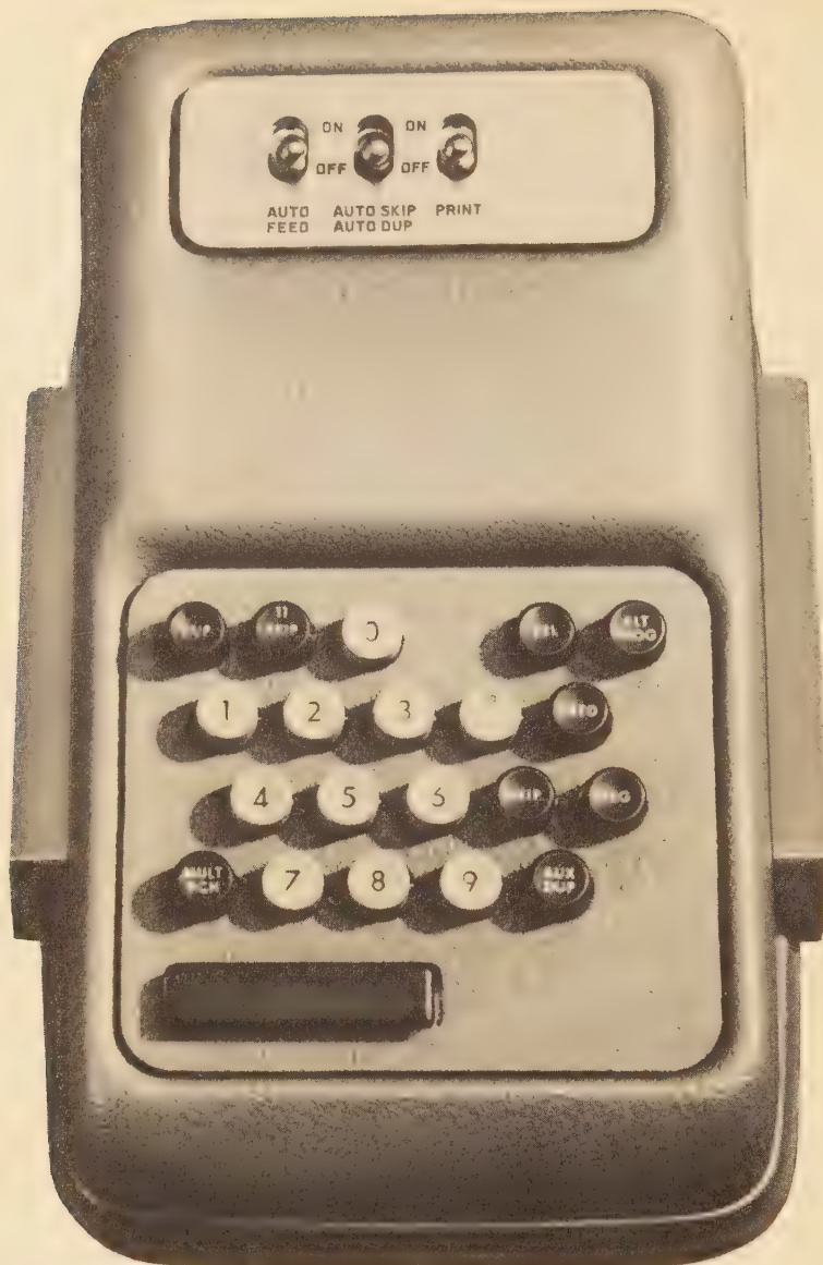
Figure 4.1 Numeric keyboard of the 024/026 card punch
