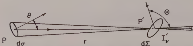
Fig. 2.4 Pencil of radiation at P' having solid angle d\omega = d\sigma \cos \theta / r^2 .
